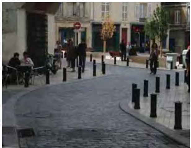
A narrow city street with the carriageway defined by bollards rather than paint
