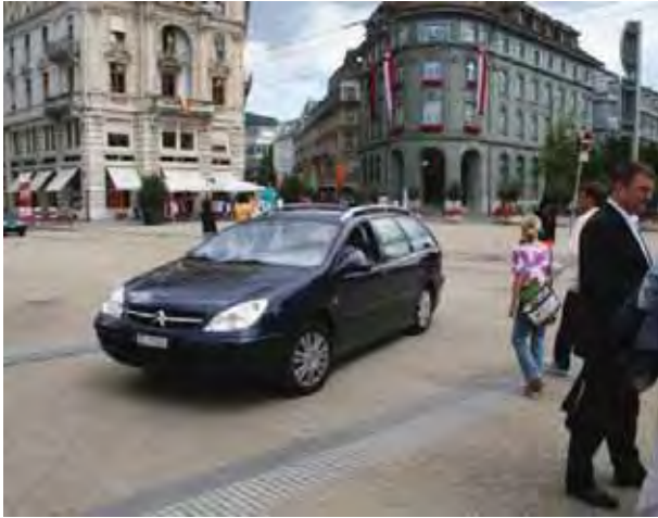
Shared Space approach to Zentralplatz, with the carriageway line defined by a different material
