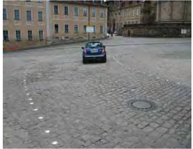
In the Domplatz, the line of the carriageway is defined by aluminium studs. There are no white lines
