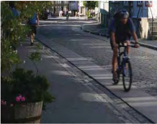
Extended pedestrian crossing with cycle lanes and one-way street all on one level
