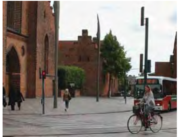
Shallow kerbs and uniform material across the space helps to reduce the impact of the motor car
