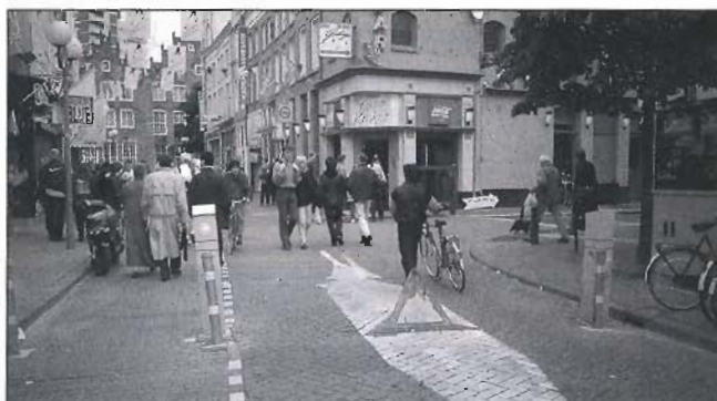
Hydraulic Bollard which restricts access for servicing. The Netherlands
